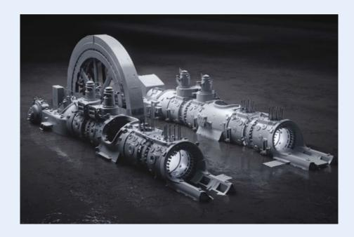
This is a huge object, an old gas turbine from a power plant in Luxembourg. Total length is 26 meters, and the flywheel is 6 meters high. Here too, a combination was made with the Ray (18 scans) and the LEO scanner (67 scans). Total project size 186 Gb of which 170 Gb was scanned with the LEO. Transferring the data alone took about 5-6 hours.
